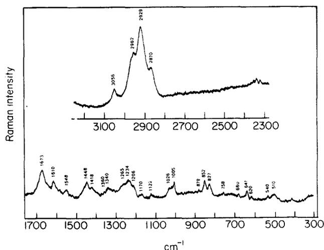
**Figure 2** Laser-Raman spectrum of the eggshell of the silkworm *Bombyx mori*. A 90° scattering geometry was employed, with the laser beam hitting the eggshell surface tangentially (outer lamellar layer). Instrumental conditions: excitation wavelength 514.5 nm; scanning speed = 10 cm<sup>-1</sup> min<sup>-1</sup>; time constant = 2 s; spectral resolution 5 cm<sup>-1</sup>; laser power at the sample = 100 mW
